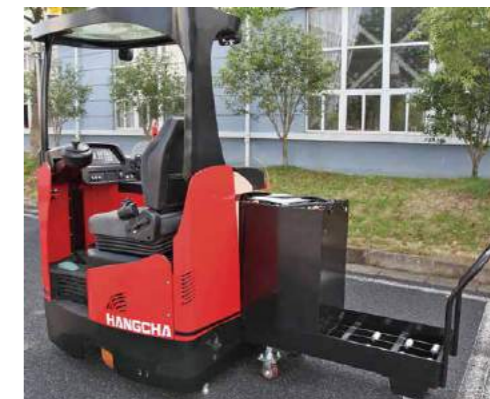
Standard configuration: Battery side roll-out + trolley(optional)
